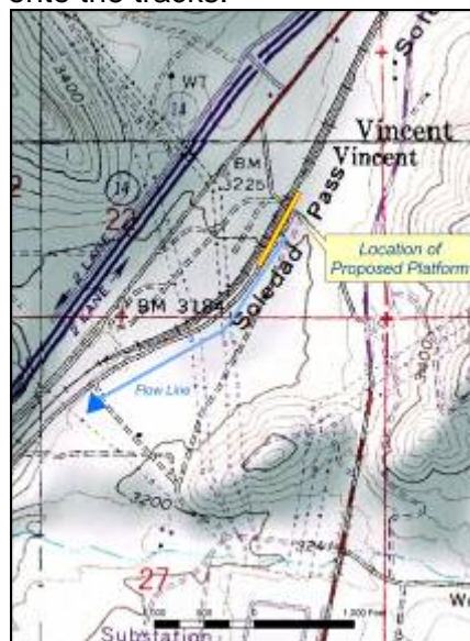
Direction of Natural Site Drainage
